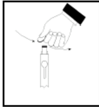
Figure 2: DO Probe Reconditioning
